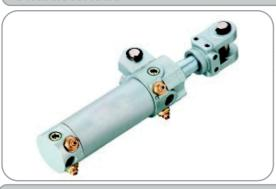
Front and rear caps are finished by aluminum alloy die-casting,processed with high precision. Three side are settled air port,easy for installation,the flow-limiting valve in front and back sides, movement speed is adjustable. Adjustable air cushion in the front and back sides, Interface of double-toggle is special designing for welder when weld the car body.
